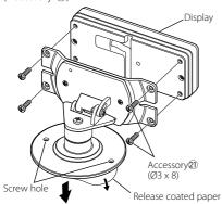
3 Remove the coated paper from the display stand (Accessory ⑦), and paste it on the mounting surface.
